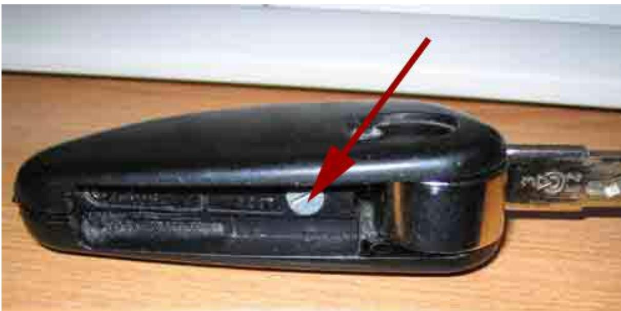
Turn the screw to Unlock and then remove the battery. You can just see the screw in this picture.
